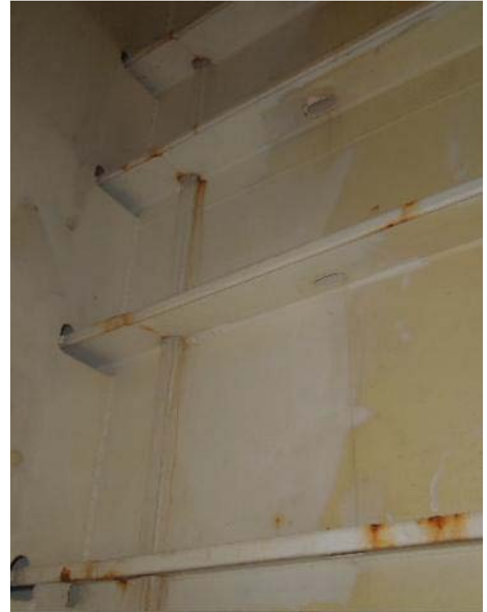
Coating breakdown starting to occur due to inadequate stripe coating on 2 year old PSPC ship
