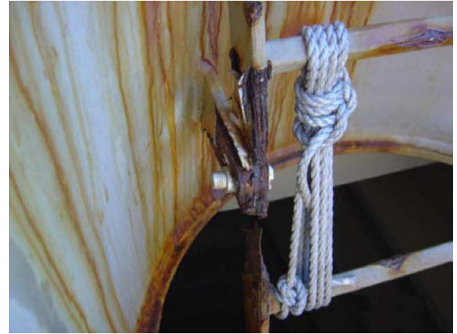
Corrosion on PMA can be life-threatening
